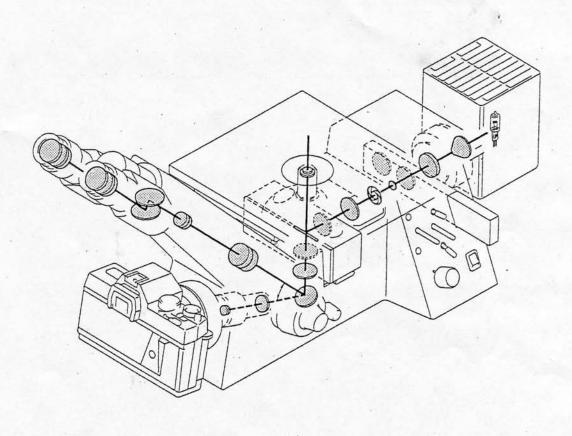
Fig 1-1 Optical design of Axiovert 25 CA
